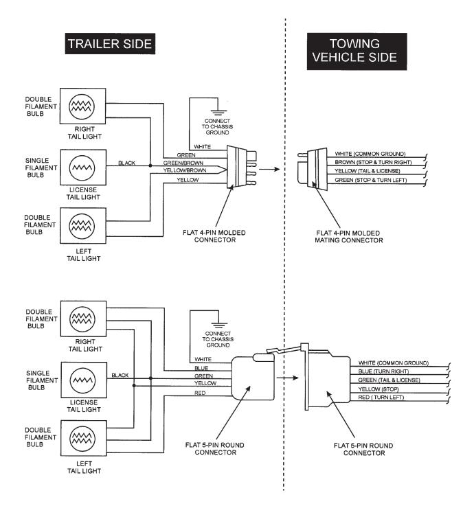
Figure 65. Trailer/Towing Vehicle Wiring Diagram
